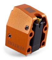
Cartridge mounting is via two threaded fixing holes utilising the supplied Vertere stainless steel thumb screws designed to ensure correct coupling of the cartridge body to the tonearm head-shell.
