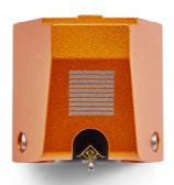
The Elliptical diamond stylus tip is rigidly fixed and bonded to an aluminium tube cantilever designed for maximum tracking ability without compromising on high frequency response or low surface noise.
