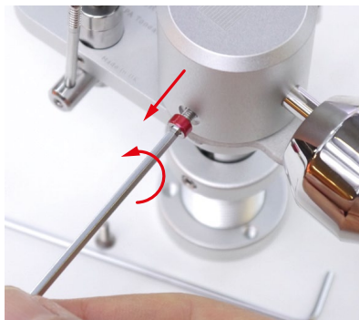
Remove Bearing Yoke Transit Screw.
